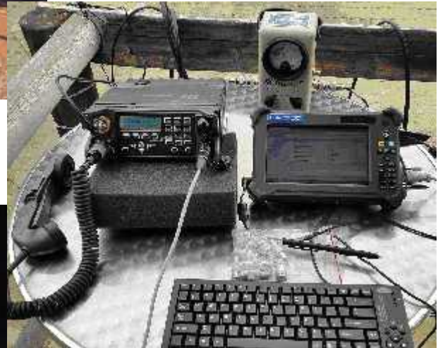
Field Testing E-mail over HF using the Leopard1 man pack radio
