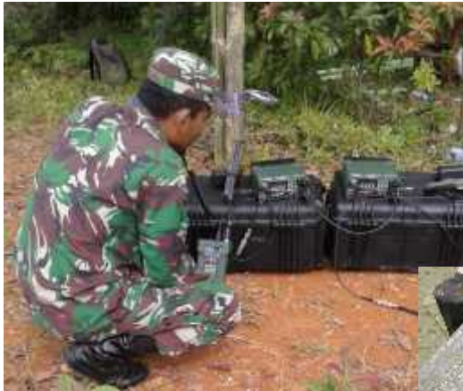
Field Testing the tactical repeater using 2 Leopard1 man pack radios
